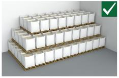
FIBCs are formed against at least two retaining walls (ie corner of a building structure), preferably three high and tiered (as with pyramid stacking).
