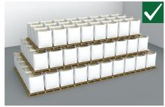
Each bag above the first level must sit on at lease four seperate lower bags. Each layer is subequently tired inwards effectively forming a pyramid structure.
